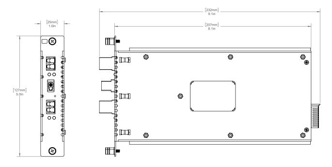
Note: DOTS and DORW models omit the bottom dual-LC/APC connector. DODC model omits the middle LC/APC connector.
